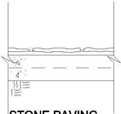
STONE PAVING On Concrete
